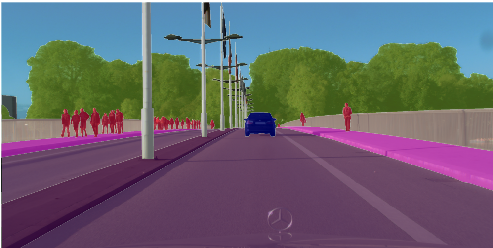
Figure 1. Example of semantic segmentation from the Cityscapes [4] dataset. Each pixel is overlaid with a color representing its class, e.g. red - human.
