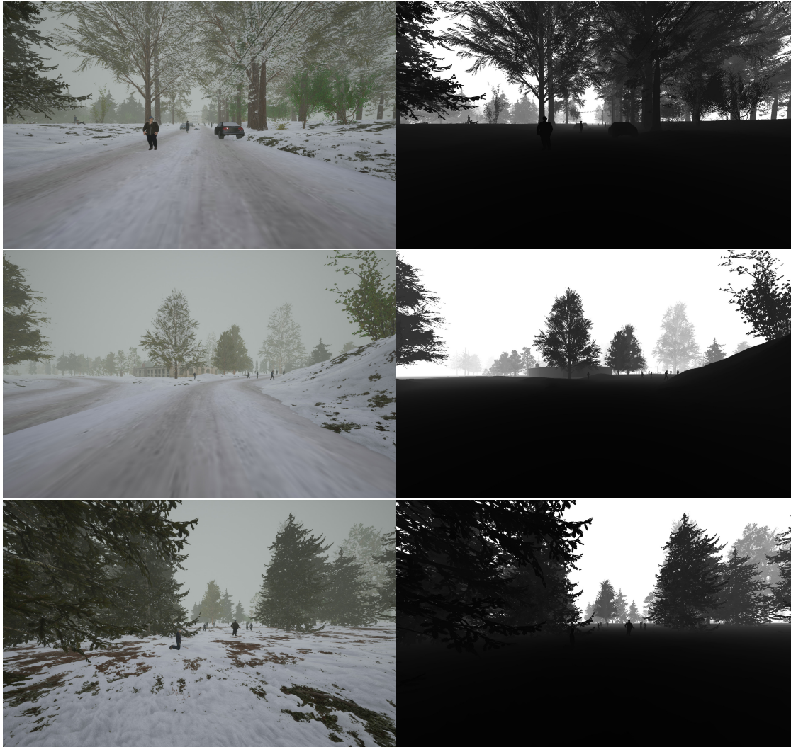
Figure 21. Examples of depth ground truth. Rows are 3 different samples. Columns are 1) the original image, and 2) its target depth ground truth. Each pixel in the depth ground truth is measured in meters from the camera in range 0–255. Brighter pixels are further away than dark pixels.
