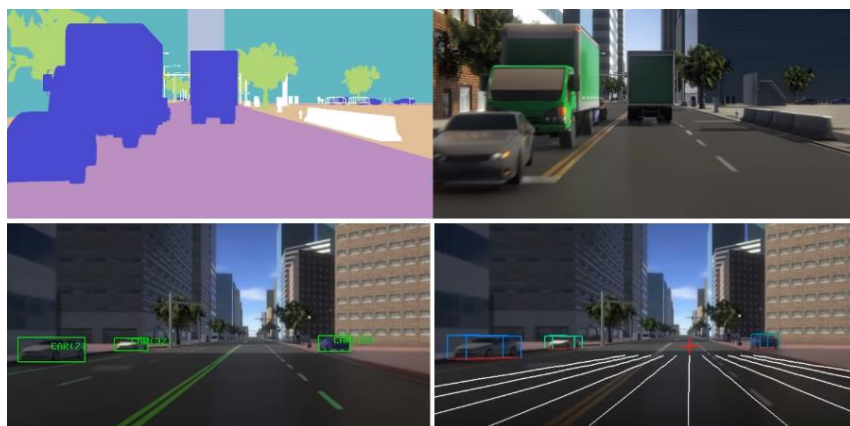
Figure 13. Example images 22 of different output labels from LGSVL simulation. Upper left: semantic segmentation (of the scene on its right), bottom left: 2D bounding boxes, bottom right: 3D bounding boxes.
