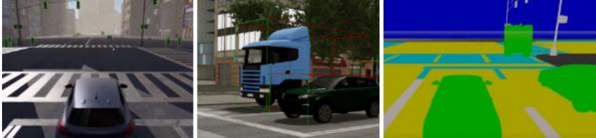
Figure 27. Output labels from the left: 2D bounding boxes, 3D bounding boxes and object segmentation.
