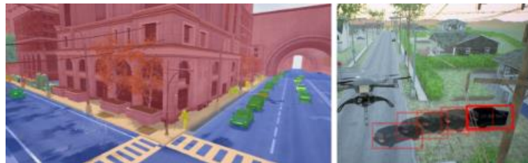
Figure 16. Examples of the output labels. From the left: semantic segmentation, 2D bounding boxes.
