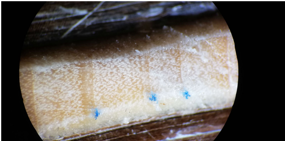
Fig. 3 An illustration of an aspen core sample where the growth rings (indicated by the blue spots) are visible
