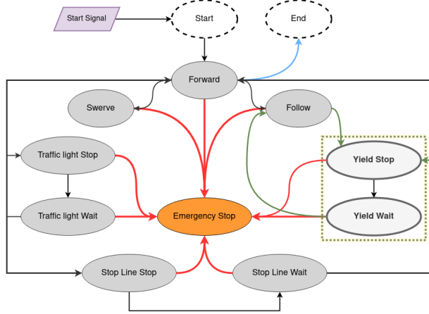
Figure 8: Behaviour state machine of AV adapted from [67] where proposed new states are shown in dotted highlighted square.
