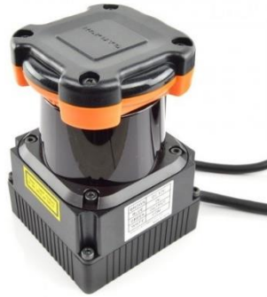
Figure 11. Hokuyo UTM-30LX Scanning Laser Rangefinder; Courtesy to [31]
