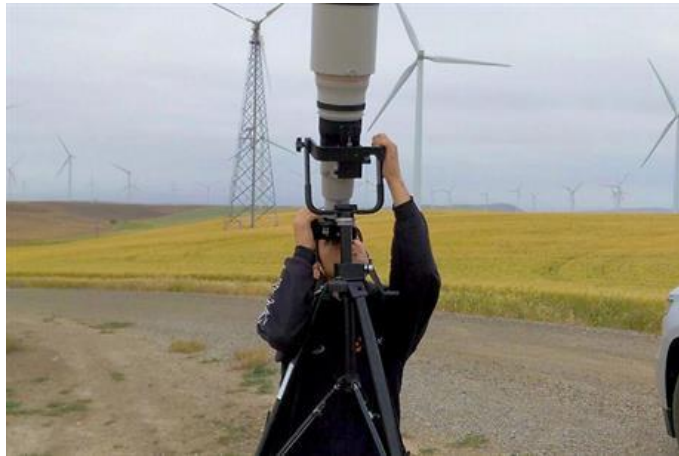
Figure 6. Blade inspection using a ground-based camera [19]
