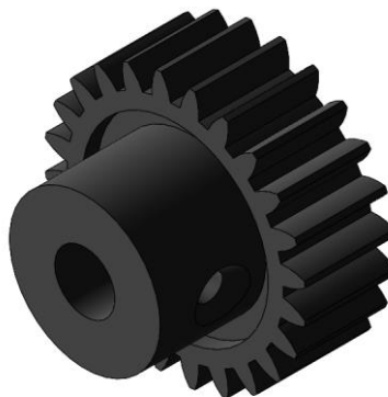
Silinderhammasratta 1M 24T mudel.
