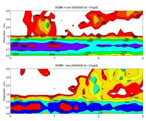
Burst of positive particles between 06:30 and 07:00 is of unknown origin.
