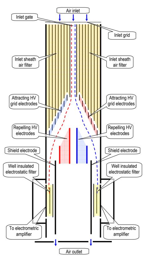
Dotted lines are two air ion trajectories. Positive ions are deflected to the left and negative to the right. Sheath air filter voltage is 520 V. Voltages of the attracting and repelling deflection electrodes are relaxing from 3000 to 25 V during every 19 second scan. Electrostatic filter collectors are supplied from 240 V internal batteries.
