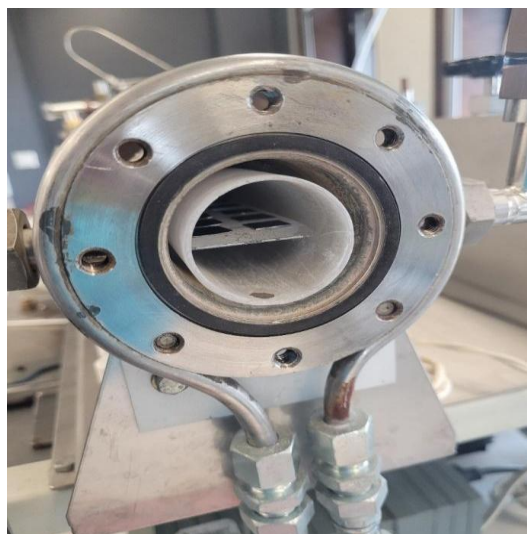
Figure 28. Samples insertion to ALD reactor, growth chamber
