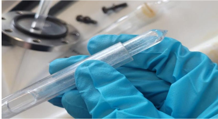
Figure 31. Tube for precursor containment inside of evaporation chamber in ALD reactor.
