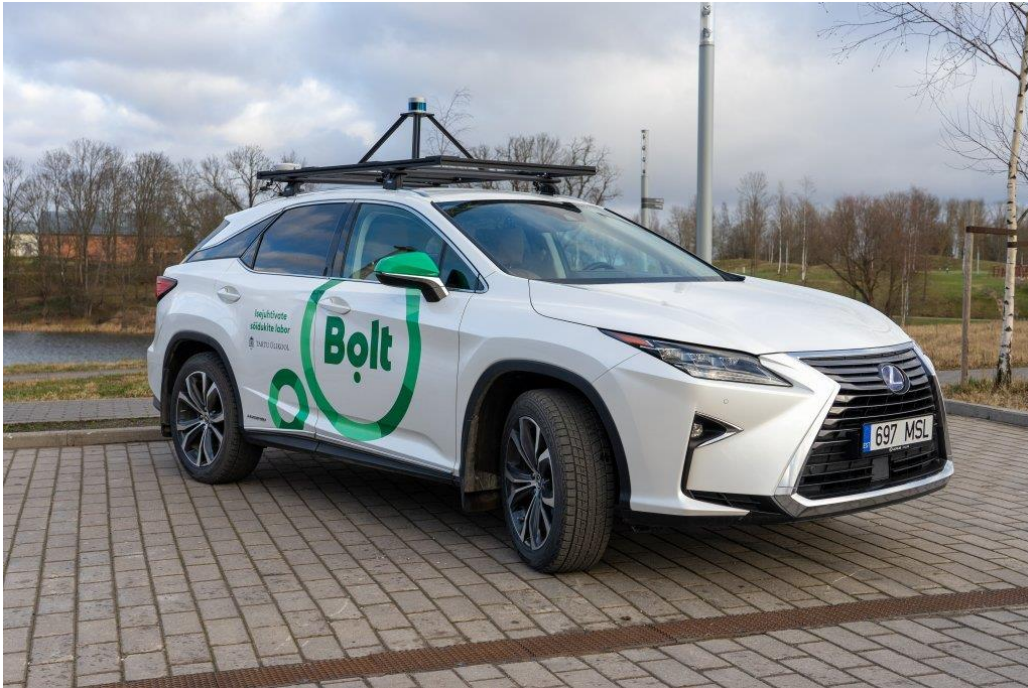
Figure 2. The Lexus RX 450h SUV used by the ADL for test drives [6].
