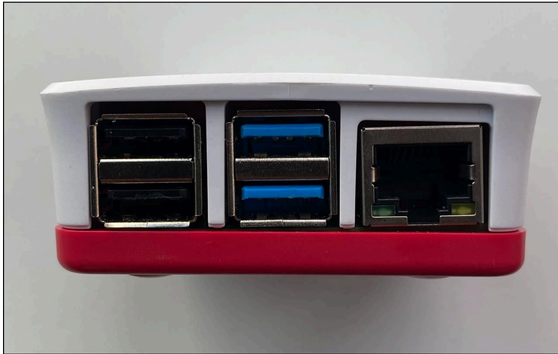
Figure 5. Real-Life View of Raspberry Pi USB Ports and Their Addresses
