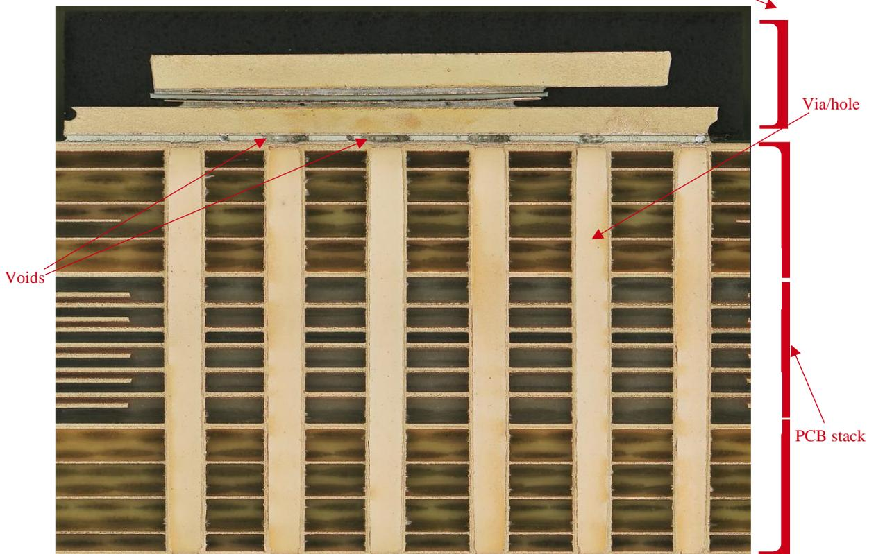
Figure 31. Cross-section overview at 140X magnification of Area 3.
