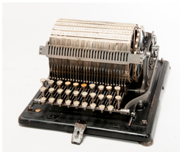
Figure 1: A photograph of the A-1 with the protective cover removed, exposing the prism with 29 alphabet strips (Häll, 2016).
