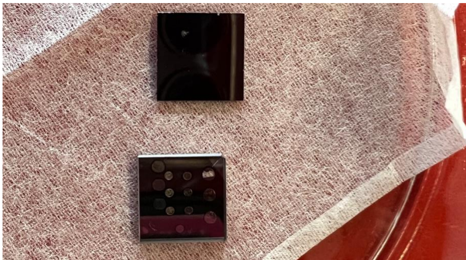
Fig. 3.1: Photograph of Si/SiO 2 substrate (above) and graphene-coated donor substrate (below).
