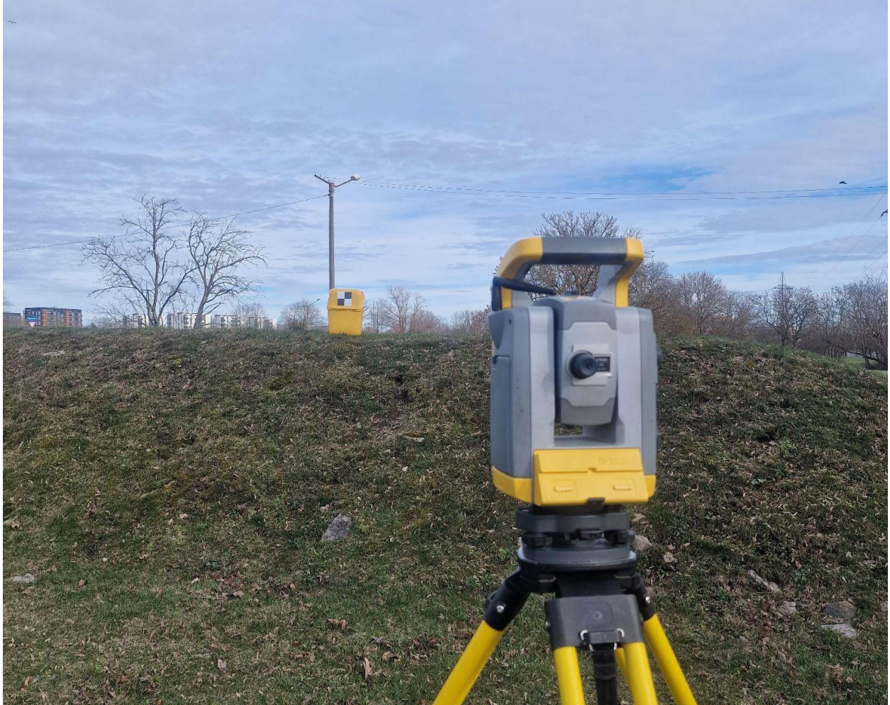
Figure 14. Marker measurement using the total station (Kevin Knjazev 2023).
