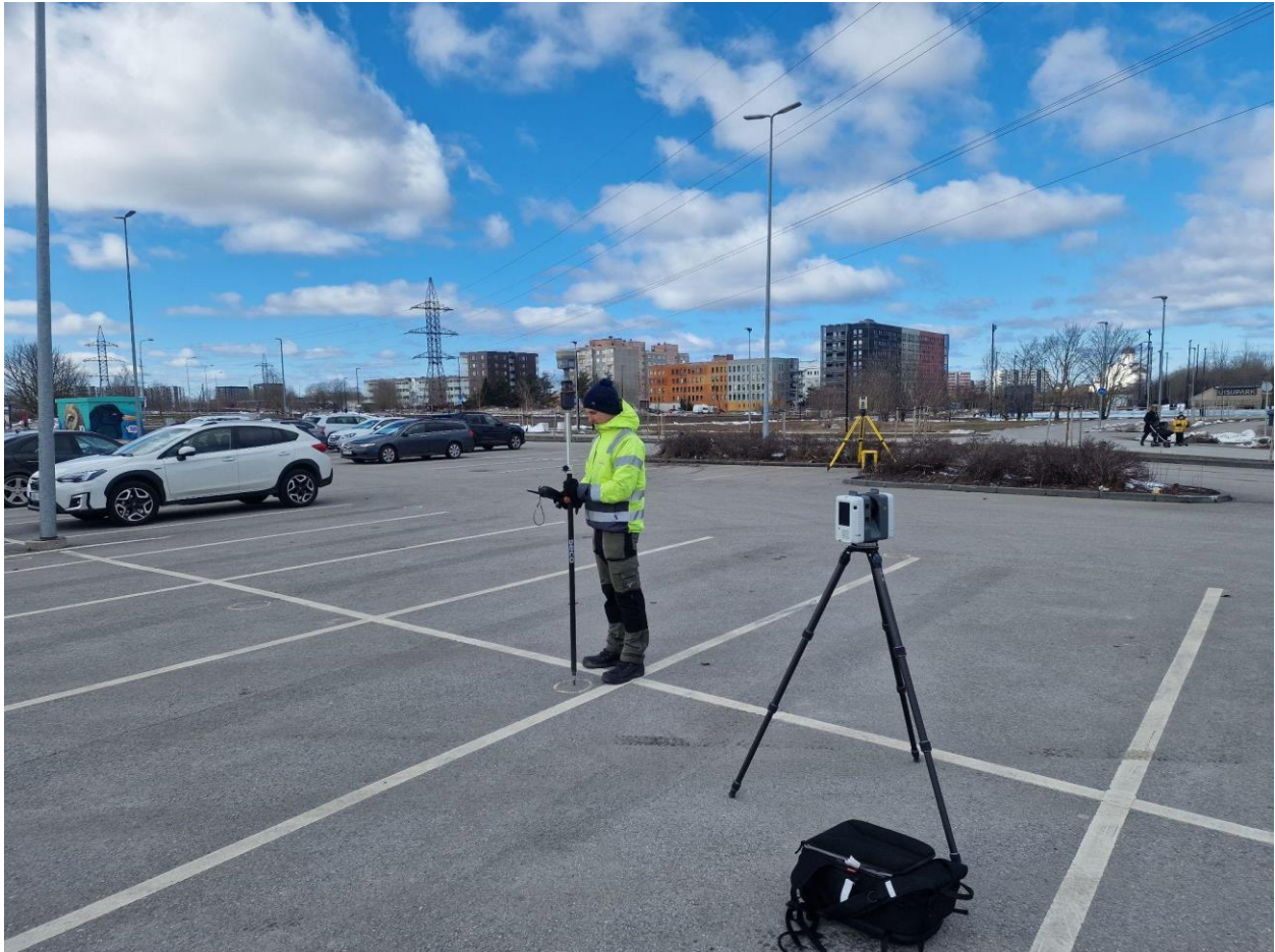
Figure 12. Photo of GNSS survey of the parking lot (Kristjan Veia 2023).
