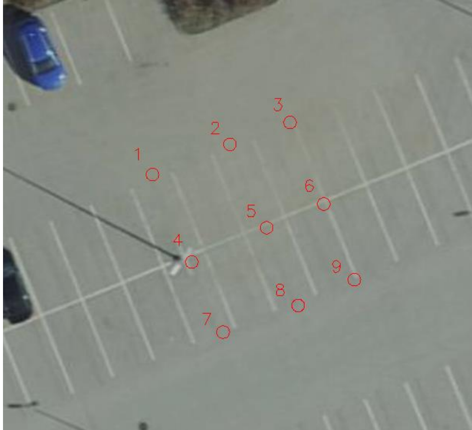
Figure 20. Point placement with orthophoto background (National Land Board).
