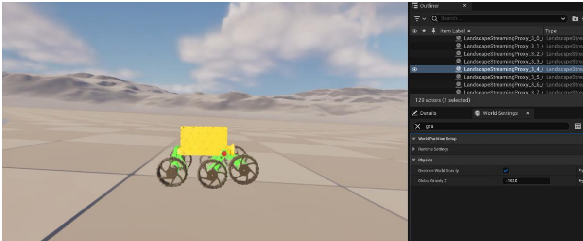
Figure 16. Digital twin’s front wheels lift from ground when accelerating in a lunar environment
