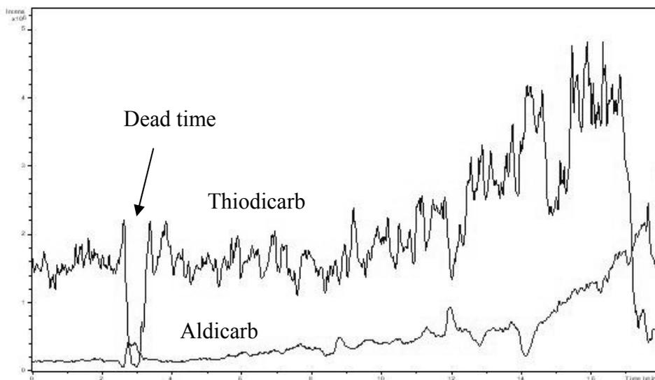
**Figure 12** MS<sup>2</sup> intensities (matrix effect profiles) for aldicarb and thiodicarb for the infusion experiment when the same extract is injected to the analytical column.
