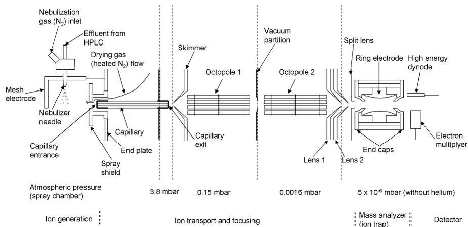
**Figure 2.** Design of the ion trap mass spectrometer with an ESI source
