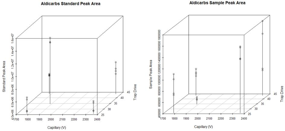
**Figure 18.** Aldicarb peak areas in standards and samples for different Capillary voltages and Tarp Drive values. In the center point other parameters were kept constant while at corner points Octopole 1 DC and Lens 2 V were changed as well.
