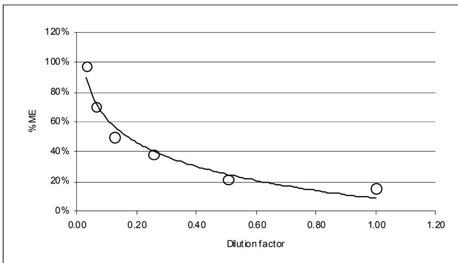
**Figure 9** Matrix effect values for methiocarb in garlic sample at different dilutions (initial concentration  $1.0 \text{ mg kg}^{-1}$ ).
