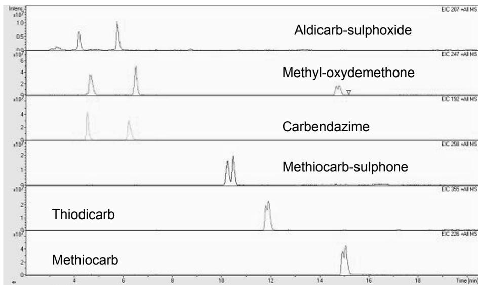
**Figure 11** Echo-peak method for 6 pesticides with gradient elution. Time between sample and internal standard injection was 1 min plus approximately 30 sec taken for completing the injection.
