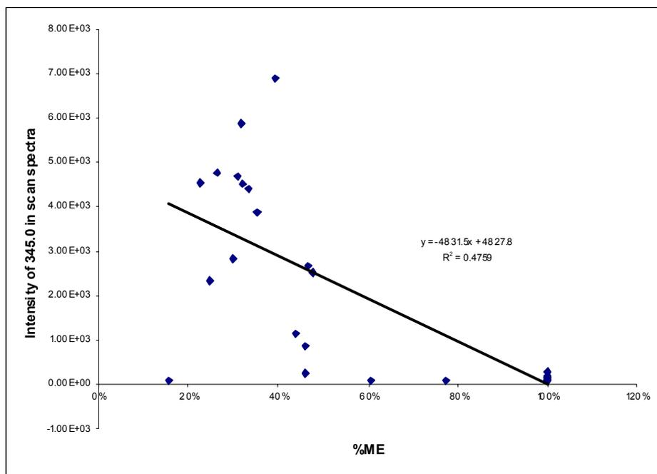
**Figure 14** The correlation plot between the intensity of ion  $m/z = 345.0$  co-eluting with the imazalil in the scan spectra and %ME values for imazalil in the same samples and standards.
