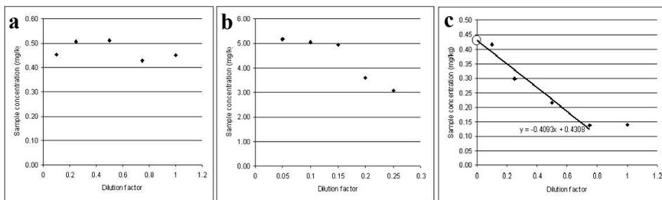
**Figure 10** Examples of different dilution plots. On y-axis an analyte concentration calculated back into the original sample and on x-axis the dilution factor is plotted. a) methomyle in rye; b) methiocarb in tomato; c) aldicarb in apple.
