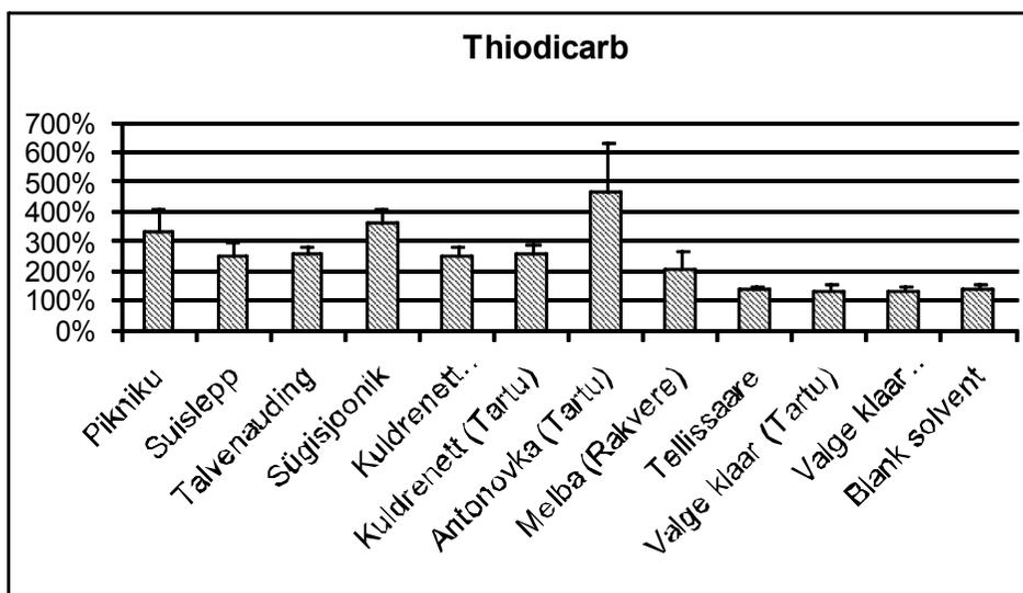
**Figure 5** Matrix effects of thiodicarb in different apple samples using the QuEChERS sample preparation method. The error bars are presented as standard deviations over 5 parallel measurements.
