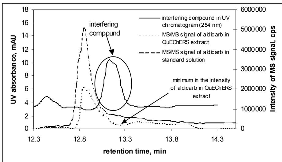
**Figure 8** MS<sup>2</sup> chromatograms for aldicarb peak in standard and in sample overlaid with samples UV chromatogram (254 nm).
