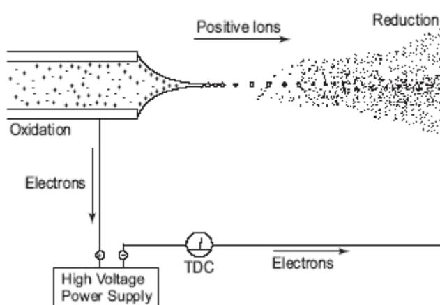
**Figure 1.** Electrospray ionisation scheme [Kearle, 2009]
