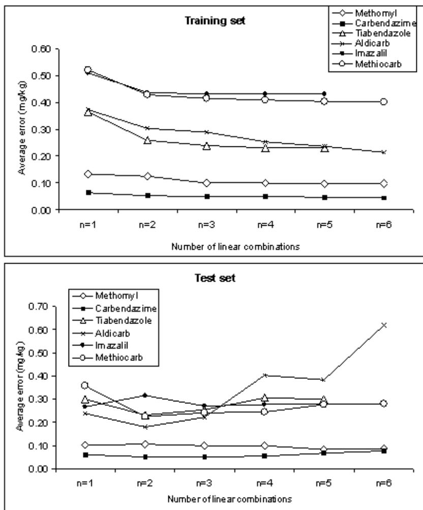
**Figure 15** Comparison of average error of predication for training set (above) and test set (below) depending on the number of components used in the PLS regression model.
