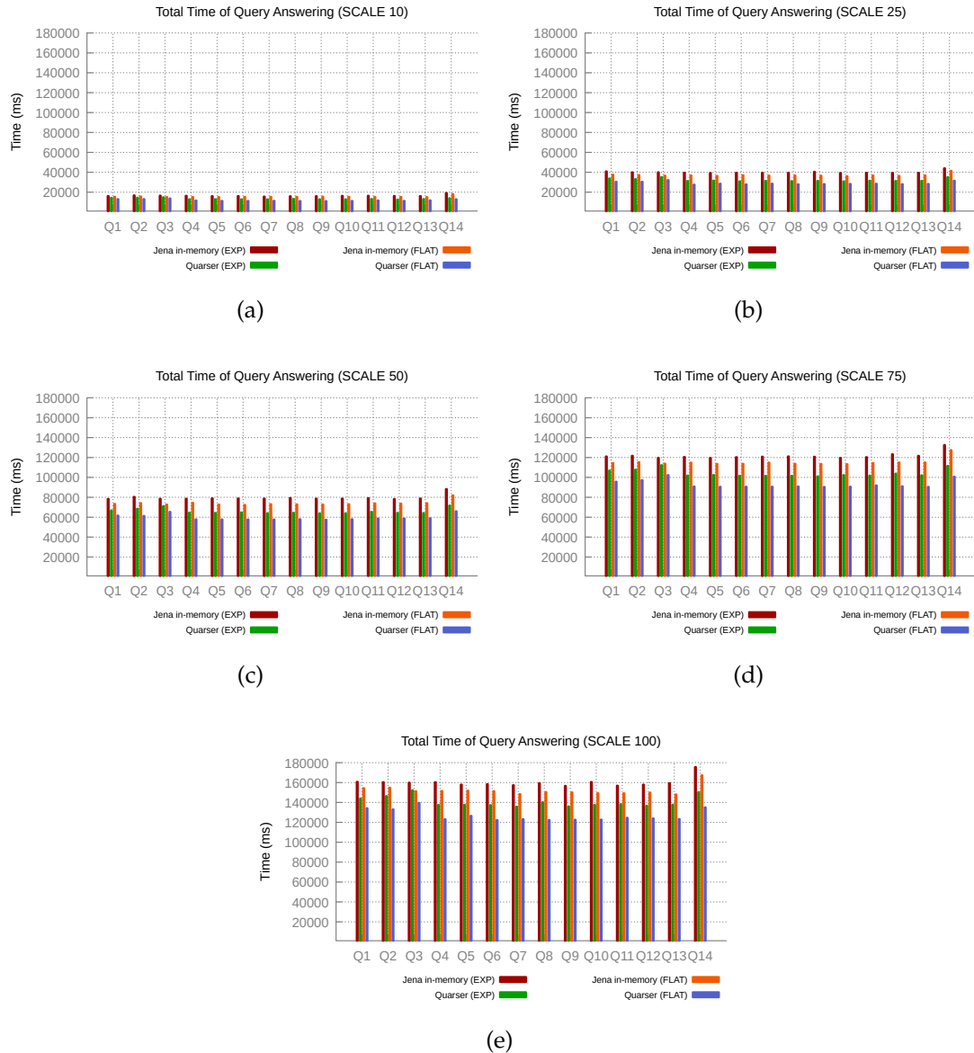
Figure 14: Total time of parsing and query of Jena in-memory vs. Quarser in Flattened and Extended JSON-LD datasets for the scales 10, 25, 50, 75, and 100
