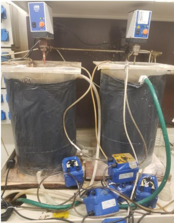
Fig. 6. View of two parallel MBBR reactors of 20 L volume based on anammox process operated at 22 °C. This project utilized just one of these reactors for PhACs removal testing (the reactor to the right).
