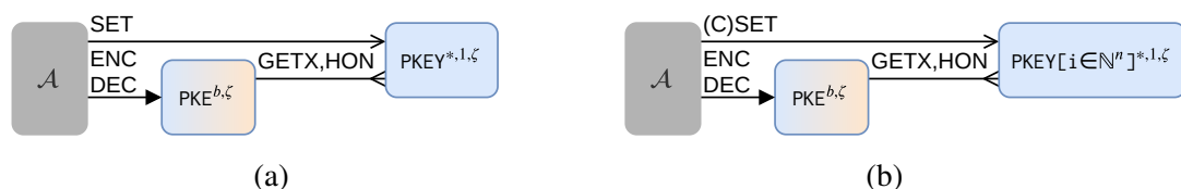
Figure 5.7: The translation of a traditional game-based definition of IND-CCA (Figure 5.6) to a package-based definition. Note that \text{GETX} := (\text{GET\_PK}, \text{GET\_SK}) .
