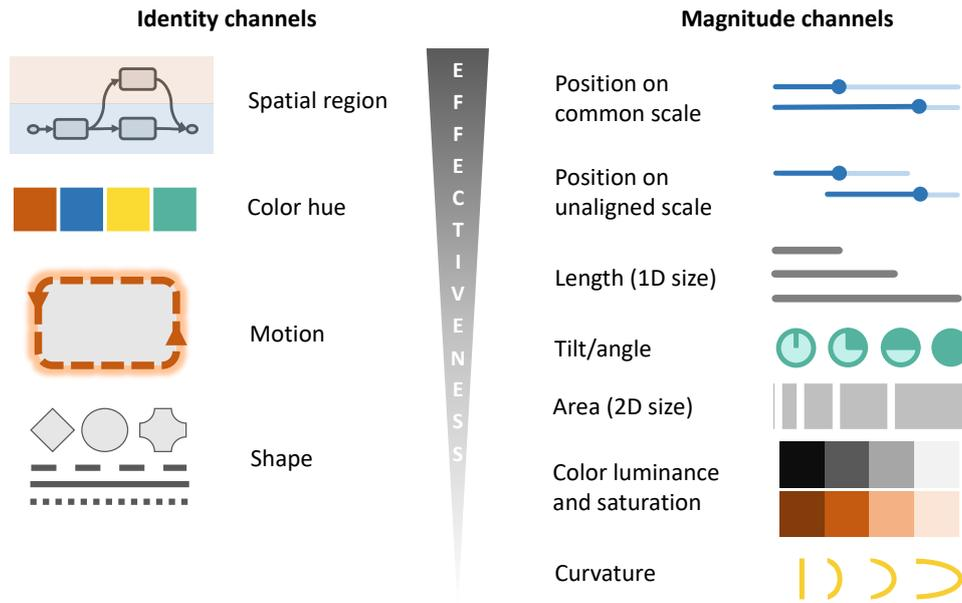
Figure 15. *Ordered attributes are visualized through magnitude channels and categorical attributes through identity channels. Channels are ordered by their effectiveness, more effective on the top and least effective in the bottom [37].*
