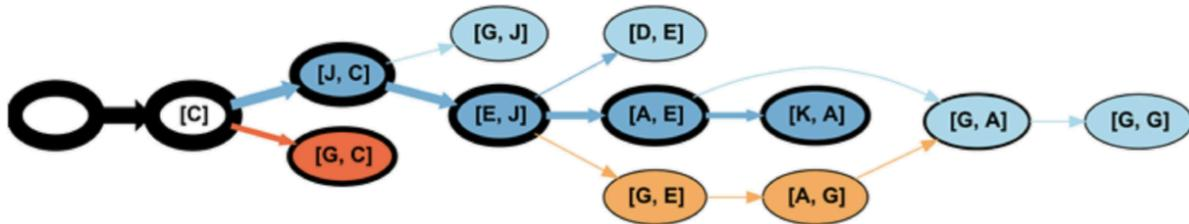
Figure 12. *Process Comparator* uses shape, size, color hue and saturation. Shapes of link endings show the direction, thickness of the links and node borders show frequency, shades of red show negative effect size and shades of blue positive effect size. Image from [2]
