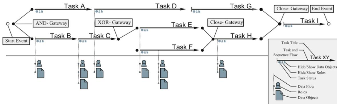
Figure 10. *Thin line diagram concept uses vertical alignment to separate process flow elements from data flow elements. Image from [6].*
