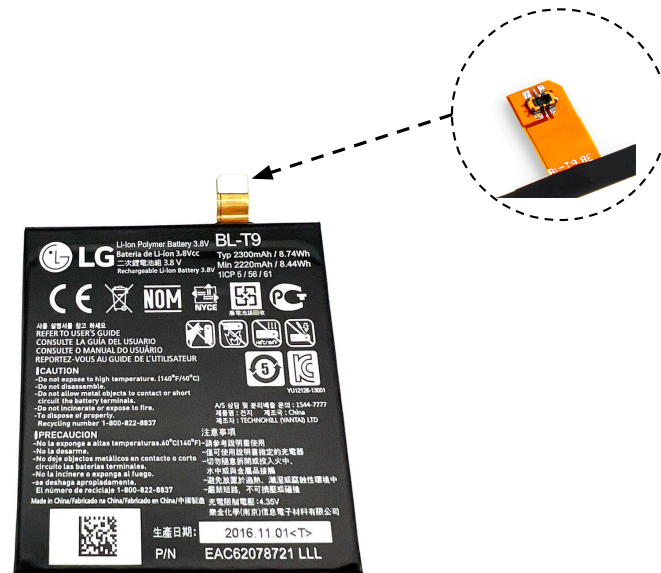
Figure 3.4: Google Nexus 5 battery BL-t9 2300 mAh.
