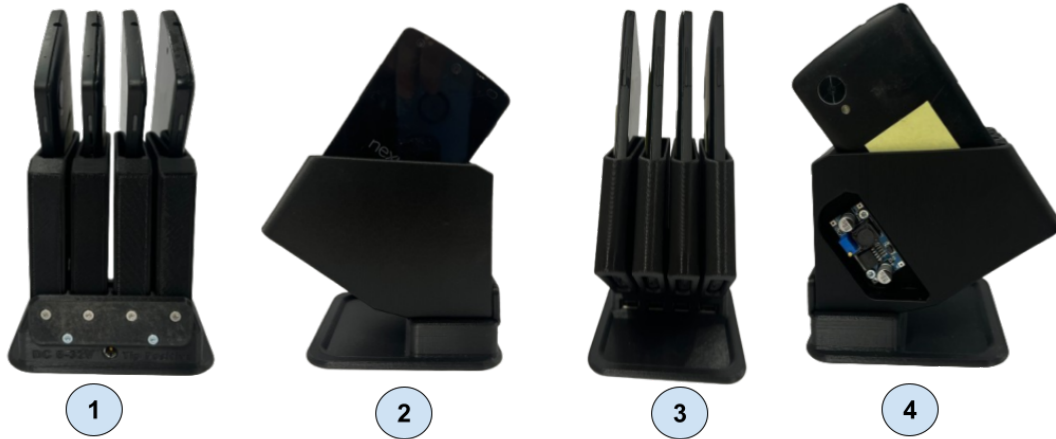
Figure 4.5: Cloudlet 3D rack prototype. (1) the back side, (2) the left side, (3) the front side, and (4) the right side.
