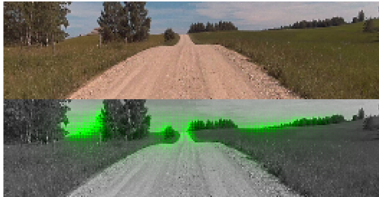
Figure 22. During steeper ascents, the horizon is lower in the cropped image causing models to concentrate on the sky and lowering predictive performance.
