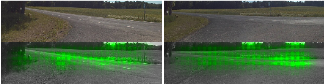
Figure 18. A difficult crossroad, where several models failed to make the turn. Left: Steering angle v1 model struggled with crossroads. Here it turned too aggressively and cut the left curb of the road. Right: Waypoints model v1 managed to complete the crossroad, although there does not seem to be much difference in the saliency map. Waypoints model seems to have better road positioning and avoids cutting the curb.
