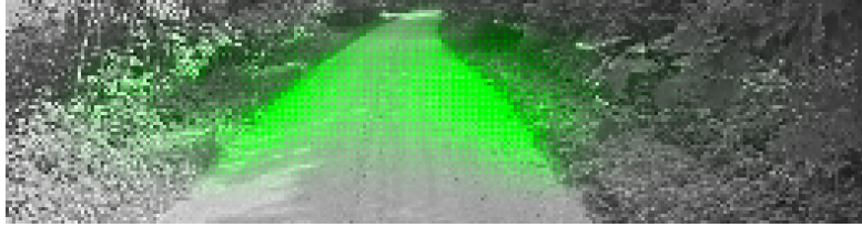
Figure 5. The VisualBackprop method can highlight salient objects of the input image.
