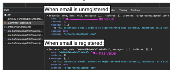
Figure 31. API response differences on the reset form of olybet.ee after an attempted fix
