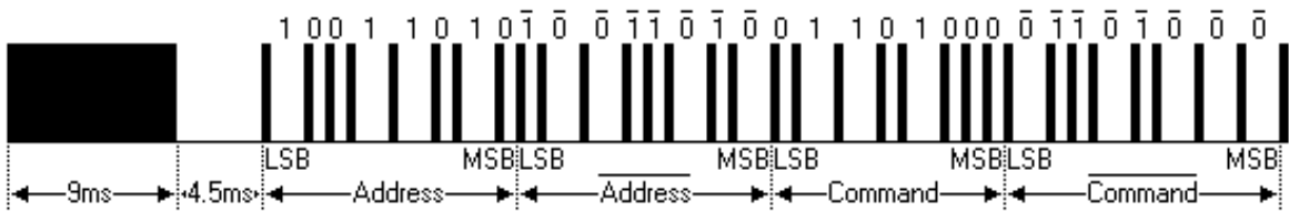
Figure 12. Example pulse stream of a NEC encoded message [30].
