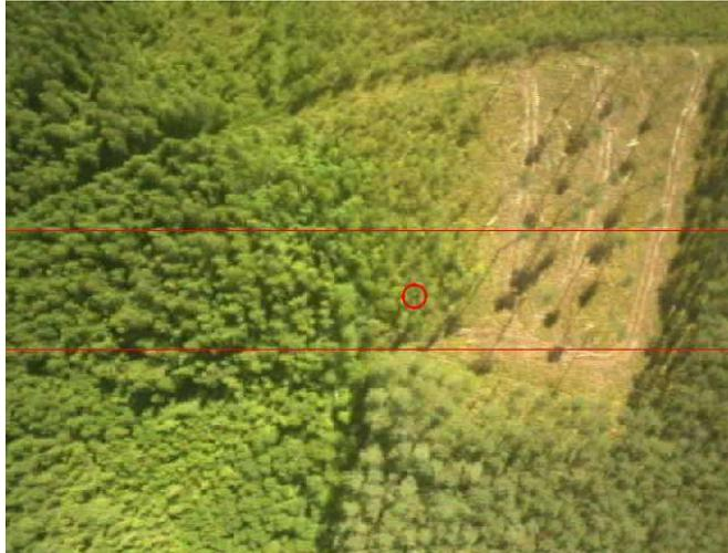
**Figure 10.** A sample UAVSpec3 web camera image. The red circle marks the footprint of the FOV of the spectrometer. Between the two red lines is the footprint of the FOV of the BRF sensor (extends over the image borders).
