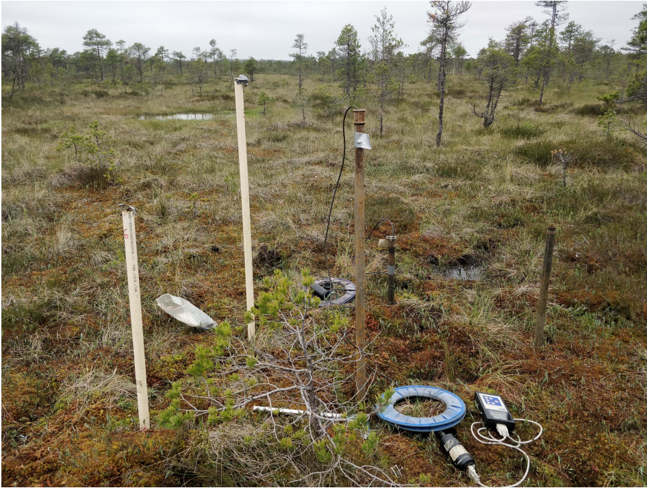
Figure 4. Measuring saturated hydraulic conductivity with BAT-permeameters and piezometer (beige PVC pipes in the picture) tests.
