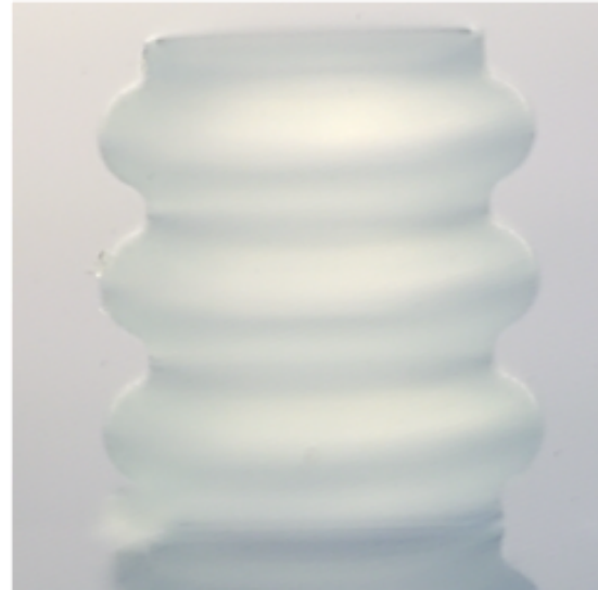
FIGURE 3.8: IP-Q bellows structure used for effective E testing.
