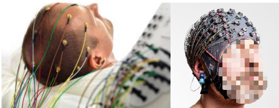
Figure 9: Technomed EEG cup electrodes (left) and cap with g.SCARABEO EEG electrodes from g.tec (right)
