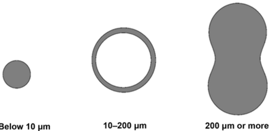
Figure 4. The effect of the initial diameter of the filament to the shape of the cured structure.
