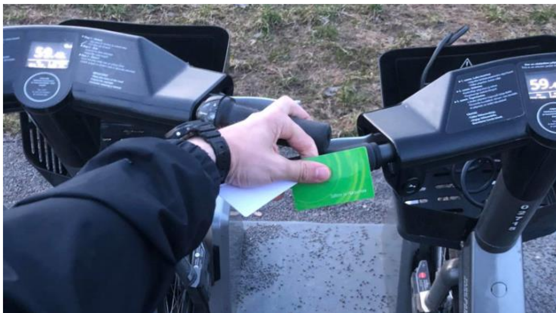
Figure 18. Two Tartu Smart Bike Share bikes unlocked at the same time with an original and a cloned card
