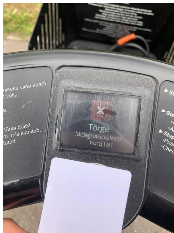
Figure 17. Using a partial clone of the Tallinn Public Transportation card
