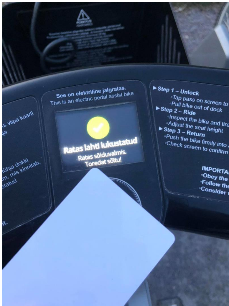
Figure 16. Using a full clone of the Tallinn Public Transportation card on a Tartu Smart Bike Share bike's NFC card reader
