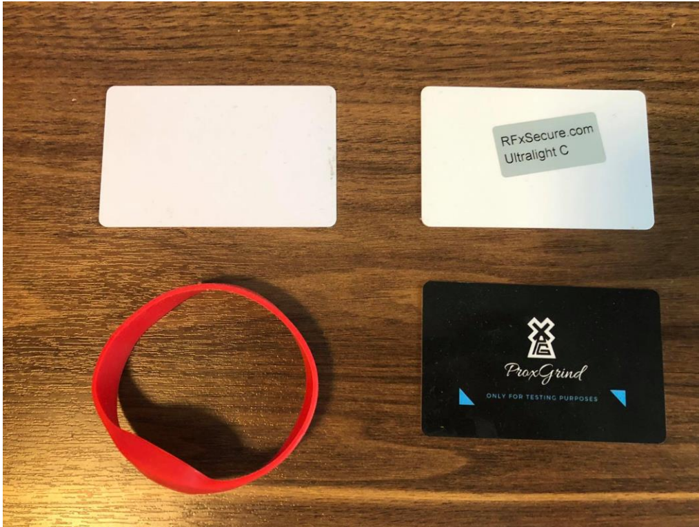
Figure 14. Top left is MIFARE Classic 1K magic card, top right is MIFARE Ultralight C magic card, bottom left is MIFARE Classic 1K magic tag, bottom right is Lab401 magic card
