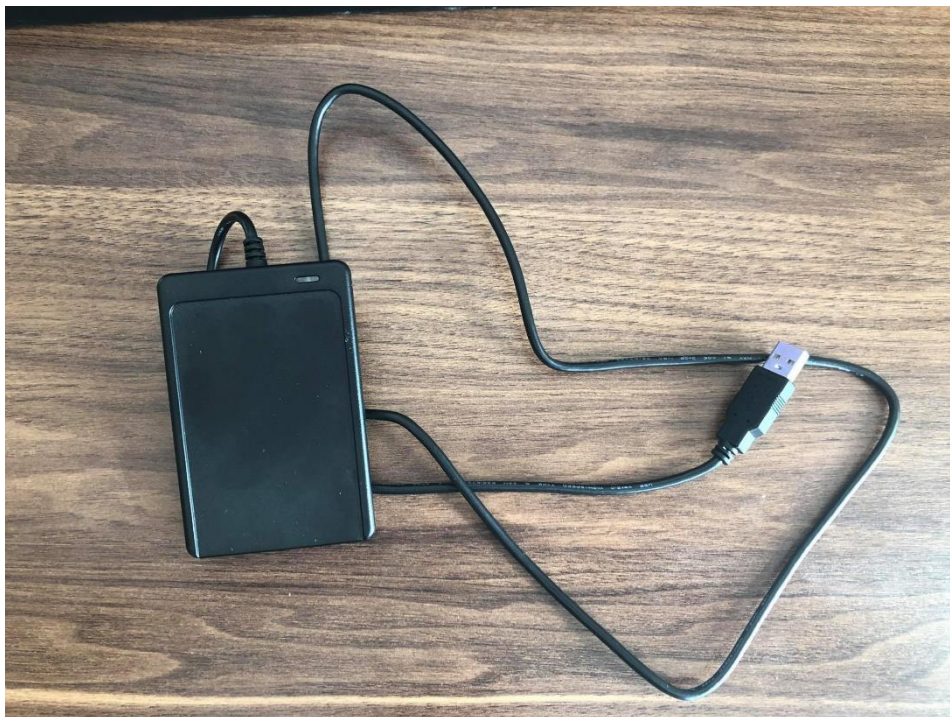
Figure 2. The ACR1252U USB NFC Reader III
