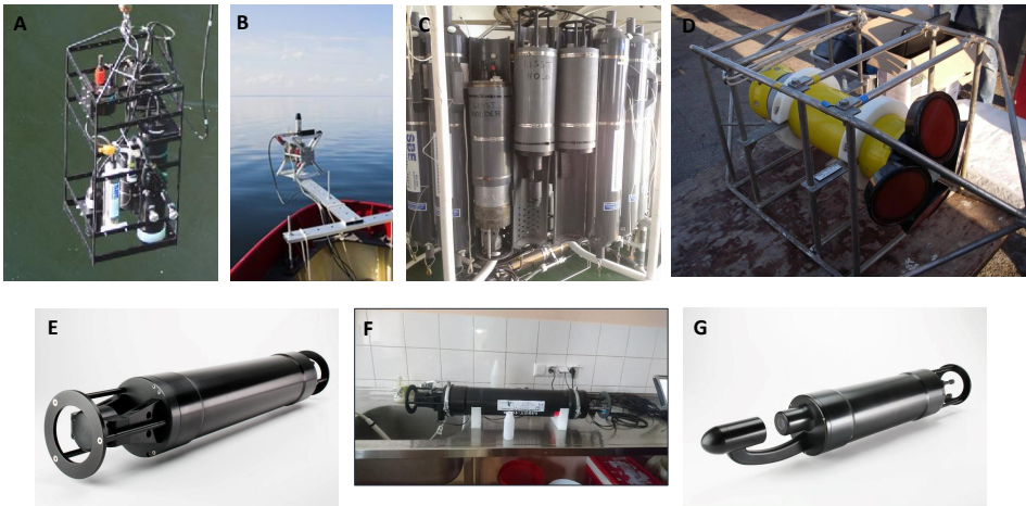
Figure 3: Instruments used during the field campaigns: A – a cage containing WET Labs AC-S, ECO-BB3, ECO-VSF3, DH-4 datalogger and Seabird CTD, B – an above-water system of three TriOS-RAMSES hyperspectral radiometers, C – a rosette containing Niskin bottles, D – 300 kHz ADCP current profiler, E – LISST-100, F – LISST-100X in a laboratory setup, G – LISST-HOLO holographic camera
