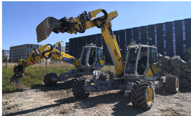
Figure 4. HEAP, the first of its kind for autonomous deployment, in front of its clone Armano, a proof of concept for teleoperated/semi-autonomous operation [6]
