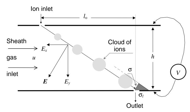
Loscertales [1998] proposed a new method improving the diffusion-limited mobility resolution by means of the longitudinal electric field in an aspiration mobility analyzer. The plain analyzer is explained in Figure. The plates of a Loscertales analyzer are not equipotential and the electric field is not perpendicular to the air flow as assumed in traditional mobility analyzers.
