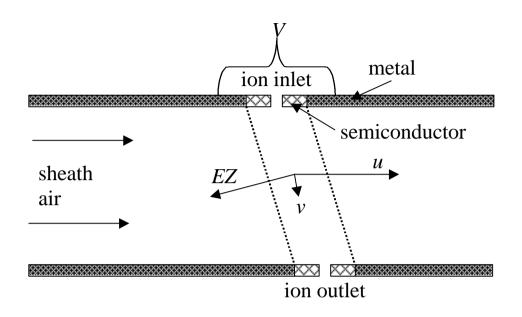
This is a modification of the Zeleny grid method. However, the configuration of fields is just the same as in a plain Loscertales analyzer.
