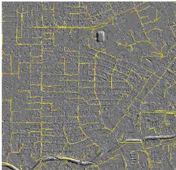
Figure 14. Flow paths from 5-meter resampled LIDAR
