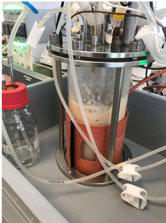
Figure S12: Foaming Problem ( in the Bioreactor)
