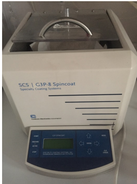
Joonis 2. Vurrkattur Specially Coating Systems G3P-8 Spincoat.
