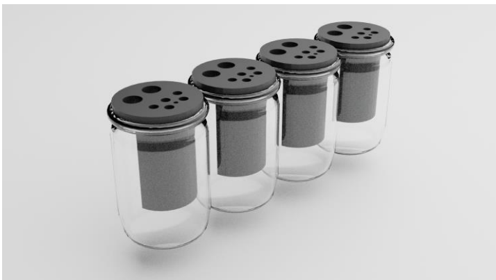
Figure 9. The design of electrochemical cells used for CFMB electrodes.
