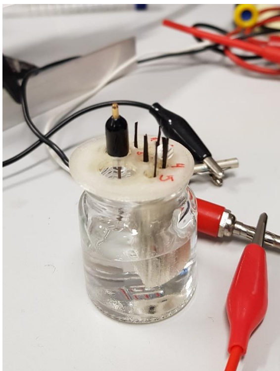
Figure 14. A photo of set-up 3D printed cell before the CV stability tests.
