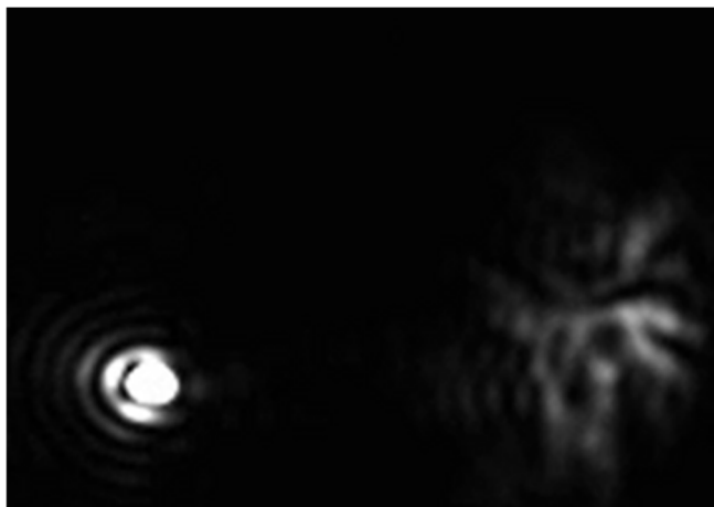
Figure 10. Captured image of the formed SrS particles (surrounded by a series of diffraction rings) in MilliQ water in the NTA video frame.
