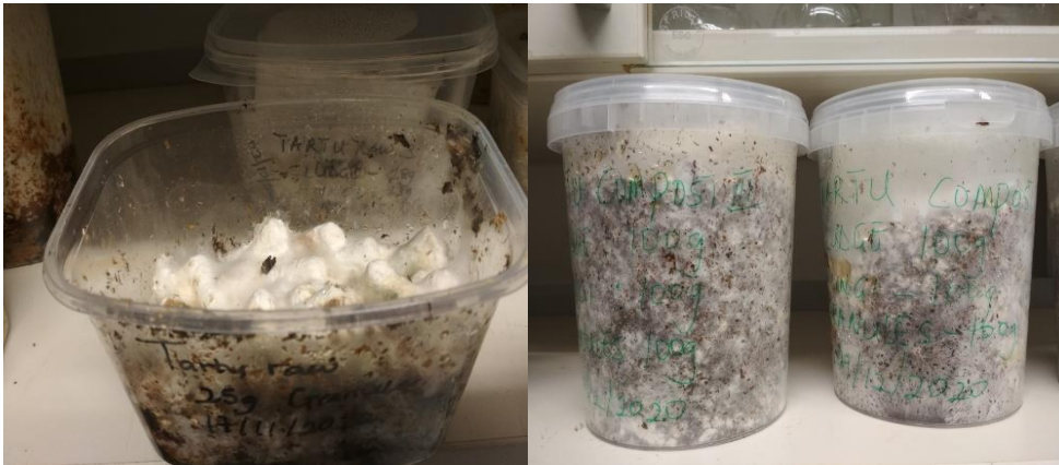
Figure 16. The result of the sterilized sludge with the combination of sludge, granules, and fungi
