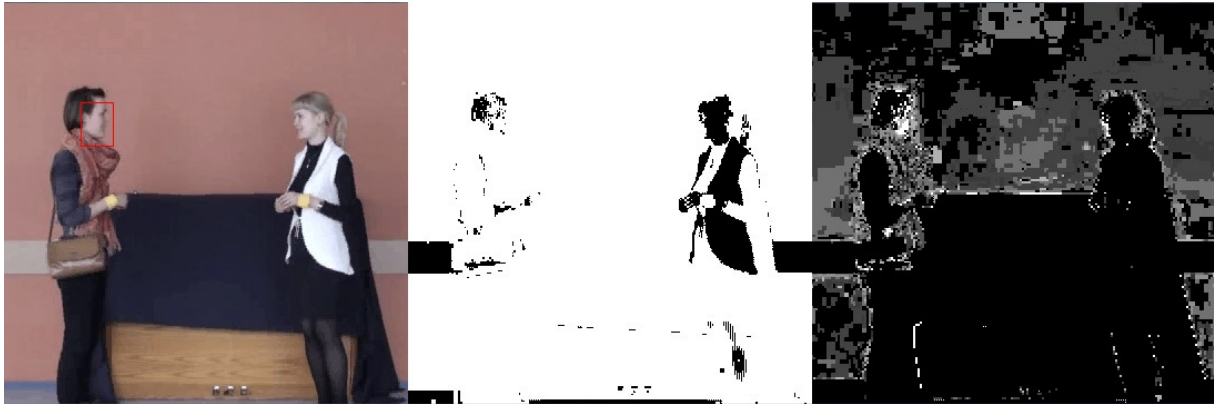
Figure 5 - normal view, saturation mask and back-projection for skin hue.
