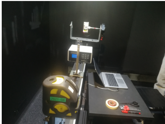
Figure 36. Using the laser to align the sensor prototype.
