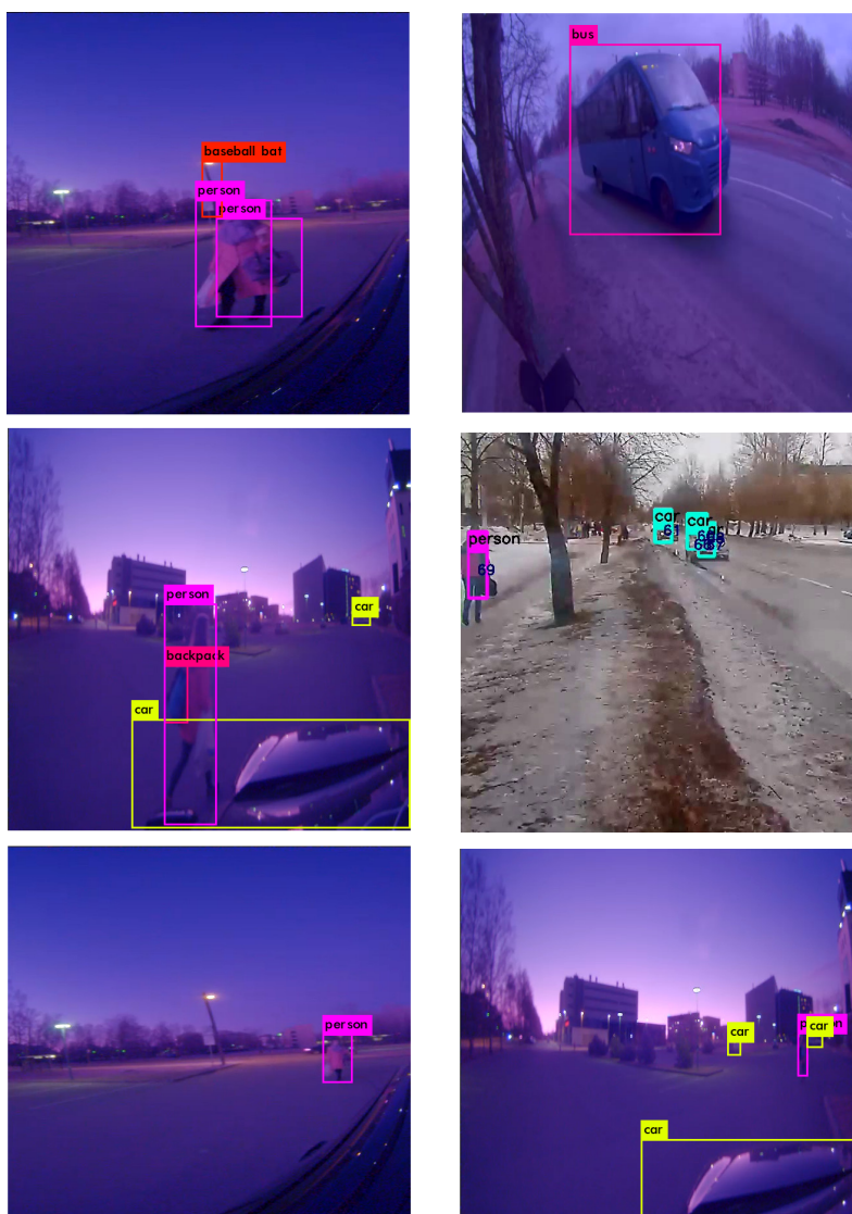
Figure 5.1: Detection and tracking examples, including low light conditions.
