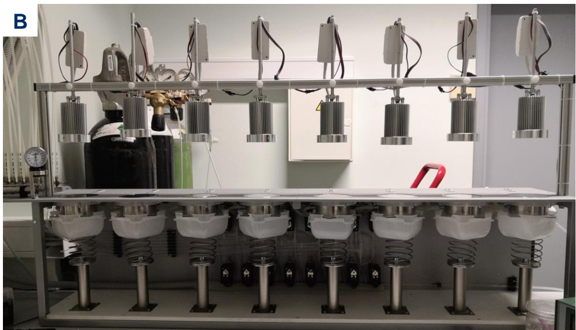
Figure 7. (A) Cuvette for A. thaliana gas exchange experiments. (Kollist et al. , 2007) (B) 8-chamber system used for gas exchange experiments.
