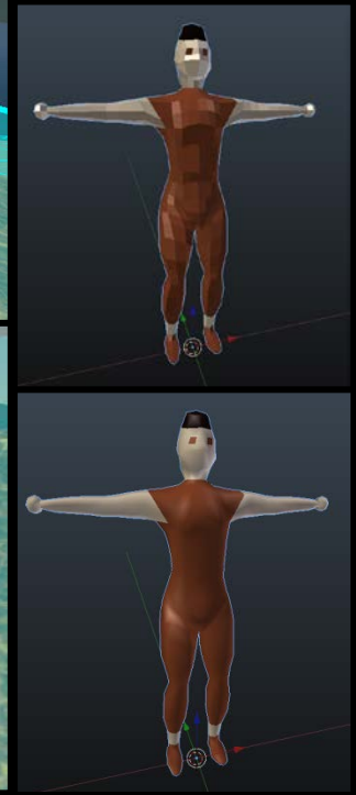
Figure 50. Flat shading (top). Smooth shading (bottom)
