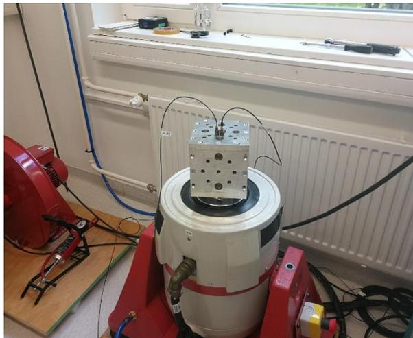
**Fig 3.10** Base test setup for a 1U cubesat.
