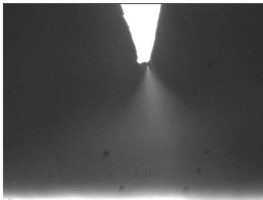
**Figure 15.** After eluent is added and its front reaches the tip of the paper visual spray is initiated. This picture is taken by a microscope attached to the nanoESI housing. The width of this picture is approximately 5 mm.
