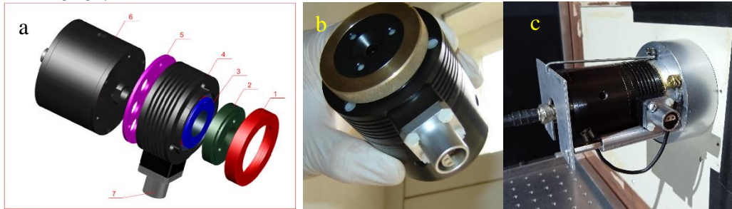
Figure 3-4 a) Schematic layout of the designed filter radiometer. The figures denote 1) brass mounting ring, 2) aperture holder with precision aperture, 3) metallic enclosure with filter, 4) metallic heater/cooler incl copper heater, plastic isolator, and Peltier' thermocooler, 5) plastic centering ring, 6) 3-Si diode trap detector, 7) electrical connector; b) Photo of the assembled filter-radiometer [14] c) installed on the monochromator.
