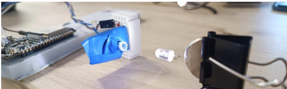
Figure 11. Prototype photogate solution with a battery powered LED. Photograph of the autor.
