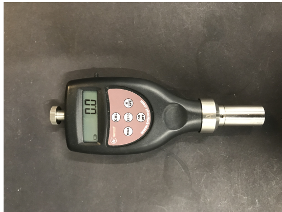
Figure 2.2: Durometer used for the experiment.
