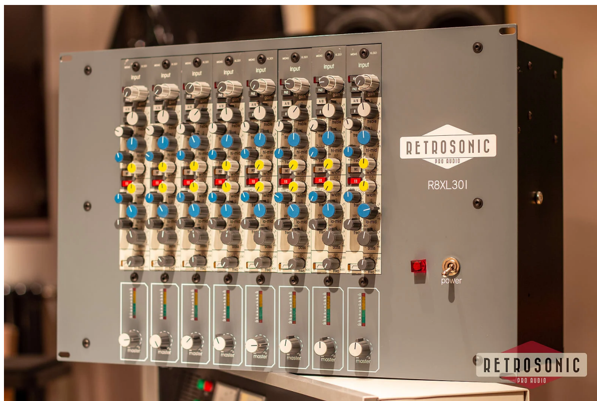
Joonis 2. Retrosonic Pro Audio R8XL301 Original Midas XL3 8-ch Mic Pre EQ. (Retrosonic Pro Audio, s.a.)
